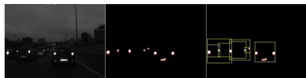
Fig. 5. From left to right: original image, individual clusters after adaptive thresholding and selected ROIs.
