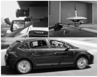
Fig. 1. Top left: Low cost stereo vision sensor. Top right: RTK-DGPS. Bottom: Experimental vehicle (modified Citroën C4).
