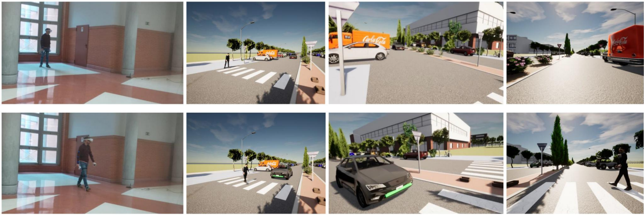
Figure 5. Pedestrian-AV interaction in VR setup. (upper row) The pedestrian waits while eHMI displays a red status. (lower row) The eHMI switches to green status and the pedestrian decides to cross. From left to right: VR experimentation environment; overview of the simulated virtual scenario; pedestrian perspective; AV perspective (simulated camera).
